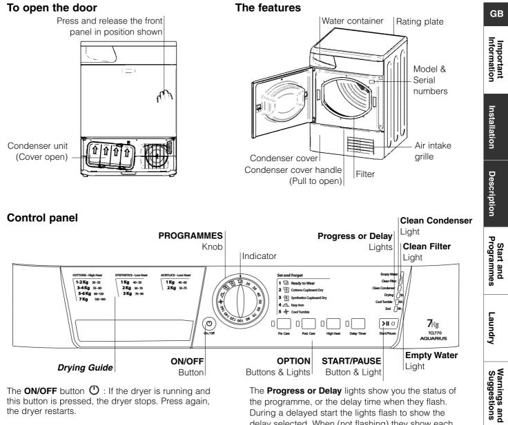
this button is pressed, the dryer stops. Press again, the dryer restarts.
